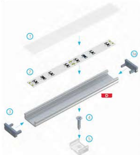
Assembly scheme for elements of the lighting system using (1) a BASIC cover, (2) a LED strip, (3) an end cap with hole, (3a) an end cap without hole, (4) a mounting screw, (5) with a D MINI mounting clip
