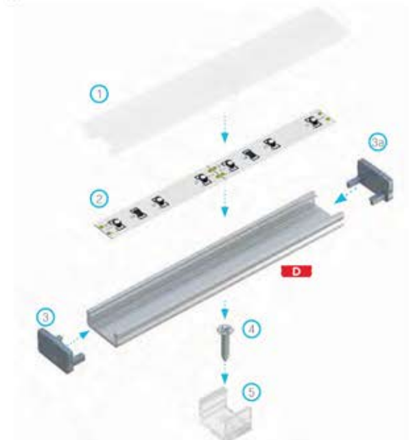
Assembly scheme for elements of the lighting system using (1) a HIGH cover, (2) a LED strip, (3) an end cap with hole, (3a) an end cap without hole, (4) a mounting screw, (5) with a D HIGH mounting clip
